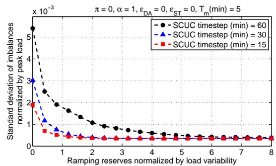
Fig. 8 The impacts of normalized ramping reserves and day-ahead market time step on the normalized standard deviation of power system imbalances [47].
