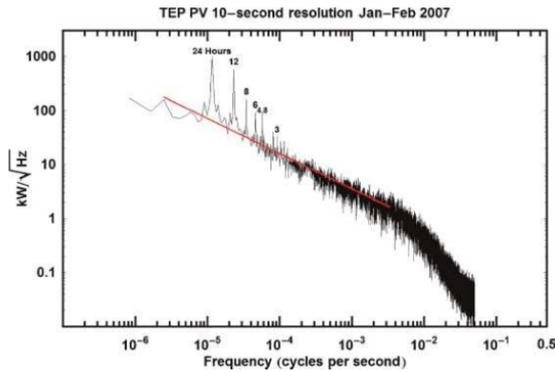
Fig. 5 Typical Power Spectrum of A Solar PV Panel [97].
