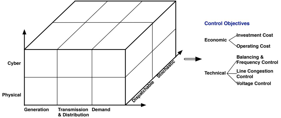
**Fig. 1** The power grid is taken as a cyber-physical system composed of an energy value chain with dispatchable and stochastic elements that must fulfill certain technical and economic objectives [32]
