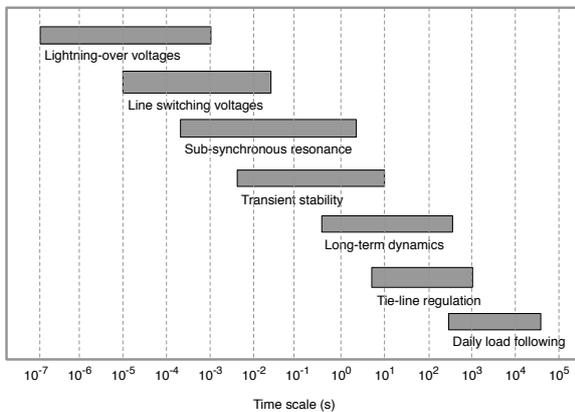
**Fig. 3** Timescales of Physical Power Grid Dynamics [95].
