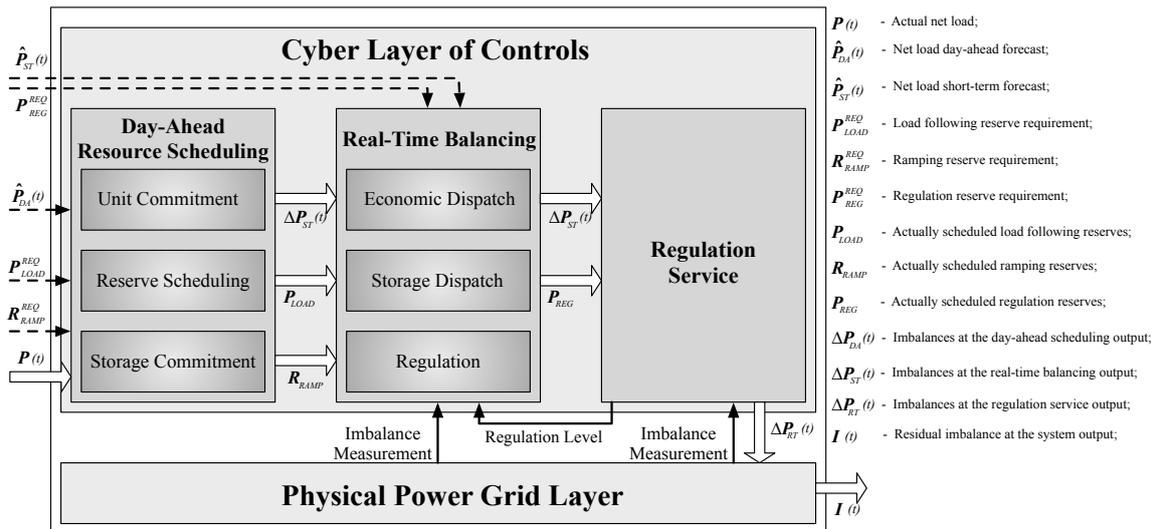
**Fig. 2** A conceptual model of the power grid enterprise control simulator [34].
