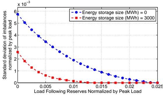
**Fig. 9** The relative trade-offs of utilizing normalized load-following reserves versus energy storage on the normalized standard deviation of imbalances [48].
