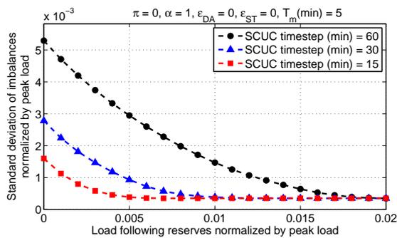
Fig. 7 The impacts of normalized load following reserves and day-ahead market time step on the normalized standard deviation of power system imbalances [47].
