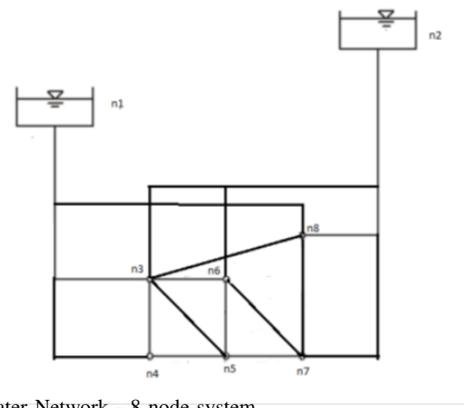
Fig. 2. Water Network - 8 node system
