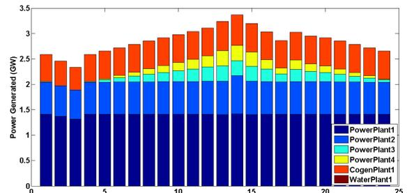
Fig. 3. Power Generation Profile over 24 hours
