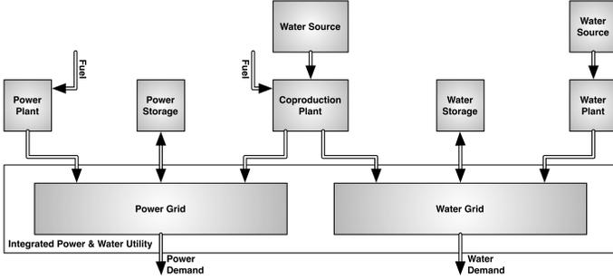
FIGURE 1. Model for the Co-Dispatch of Power and Water Supply
