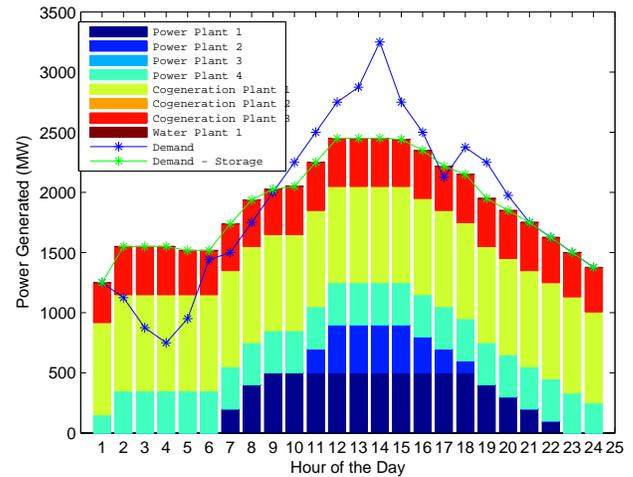
**FIGURE 2.** Base Case, Power Generation and Demand Profile Over 24 Hour Period
