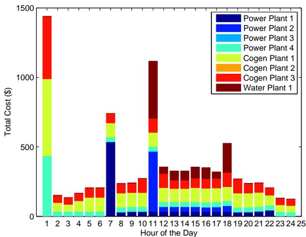
**FIGURE 4.** Base Case, Total Production Cost over 24 Hour Period.
