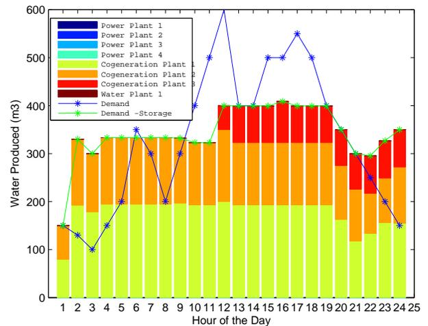
**FIGURE 8.** Middle East Inspired Case, Water Production Over 24 Hour Period
