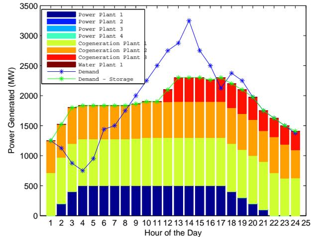
**FIGURE 7.** Middle East Inspired Case, Power Generation Profile Over 24 Hour Period
