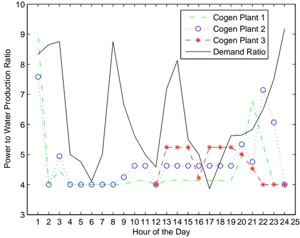
FIGURE 9. Cogeneration Plant Power to Water Ratios
