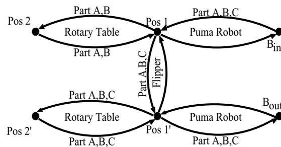
Figure 6. Robot Work Cell Material Handling Node Diagram
