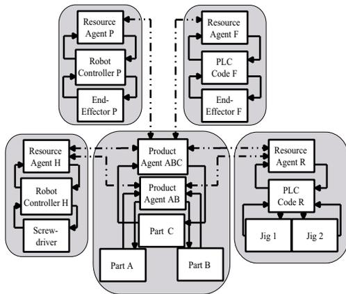
**Figure 7. Robot Work Cell Detailed Hierarchical Block Control Diagram**
