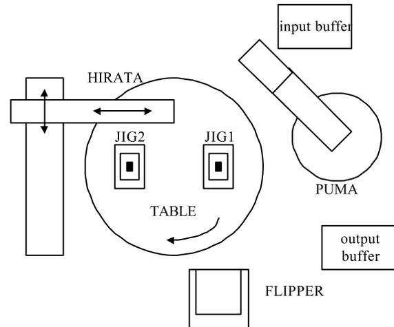
Figure 5. Schematic Diagram of the Robot Work Cell
