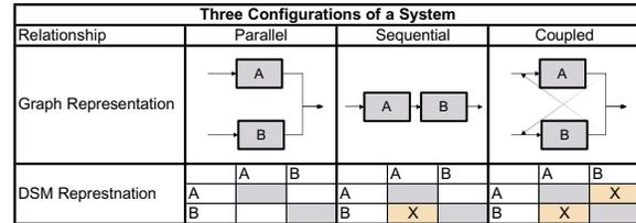
**Figure 2. DSM Representations of System Configurations**
