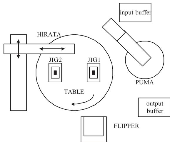
Fig. 4. A Schematic Diagram of the HCBA Robot Work Cell
