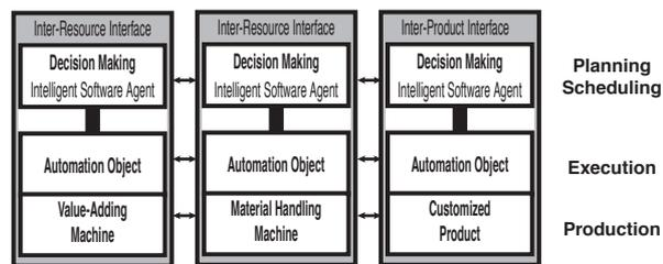
Fig. 1. A Conceptual Representation of a Distributed Manufacturing System
