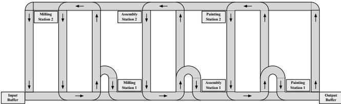
Figure 2: Starling Manufacturing System Overview [24]
