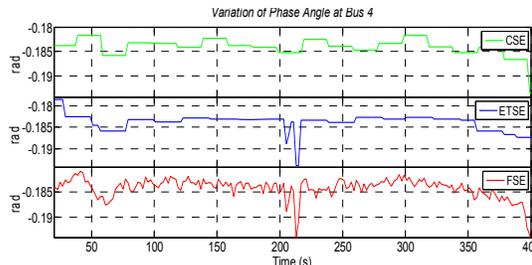
Figure 4: Variation in phase angle at Bus 4 when Bus 2 and Bus 6 have VER connected
