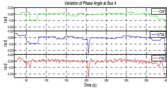
Figure 3: Variation in phase angle at Bus 4 when Bus 2 has VER connected
