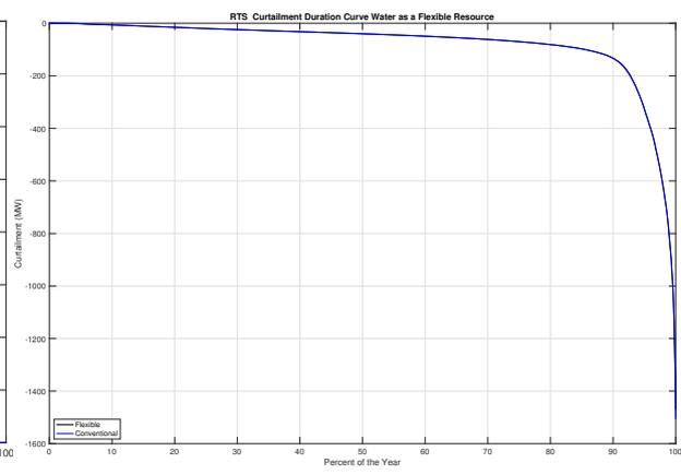
Figure 10: Curtailment Duration Curve for RTS-GMLC
