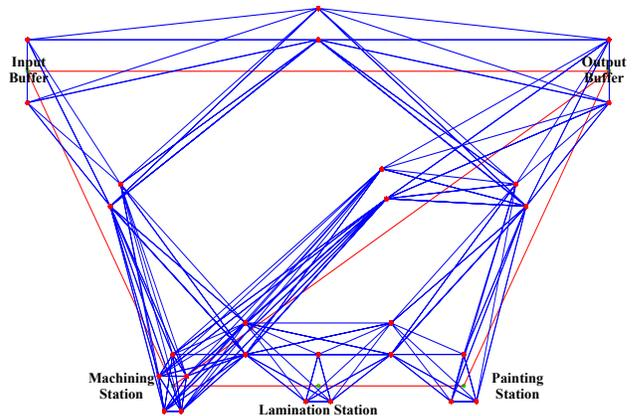
Fig. 6. Traditional (red) & Structural Degree of Freedom-based (blue) Graphs for Starling Manufacturing System in Phase I.
